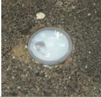
transponder in slatted floor
